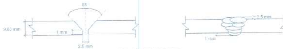
Groove Design of Test Coupon
